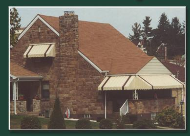
Custom made pan and cover style awnings are constructed of heavy gauge aluminum with baked enamel finish pans. Each of our thirteen available colors is white on the opposite side to reflect light. Each awning is built on a frame of the finest tempered aluminum. With a snow load capacity of 54 pounds per square foot, our awning is one of the strongest in the industry.
